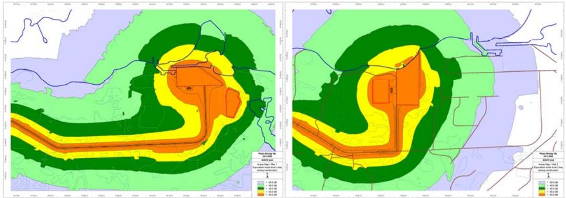
**Figure 5.7-1. Noise map for Site No. 1 and Site No. 2 during construction phase.**
