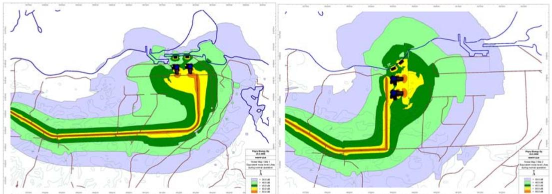
**Figure 5.7-2. Noise map for Site No. 1 and Site No. 2 during operation phase.**
