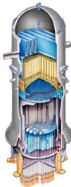
Figure 5.2-3. Schematic of the reactor core of the ABWR ( www.gepower.com/prod_serv/products/nuclear_energy/en/new_reactors.htm ).
