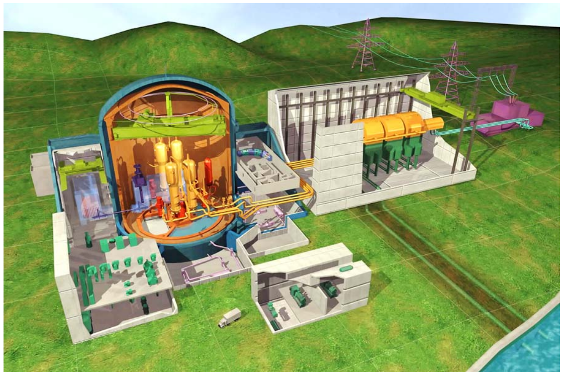
Figure 5.2-1. Schematic of the principal buildings of an EPR ( www.aveva-np.com ).
