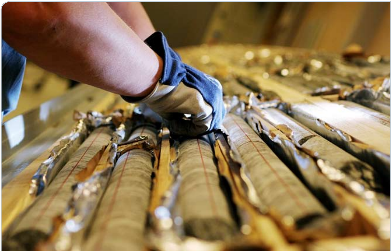
Figure 9-9 The properties of bedrock are investigated, among other things, by drilling cores. Thousands of metres of drilling samples obtained from the bedrock in Olkiluoto will be examined ( Posiva ).
