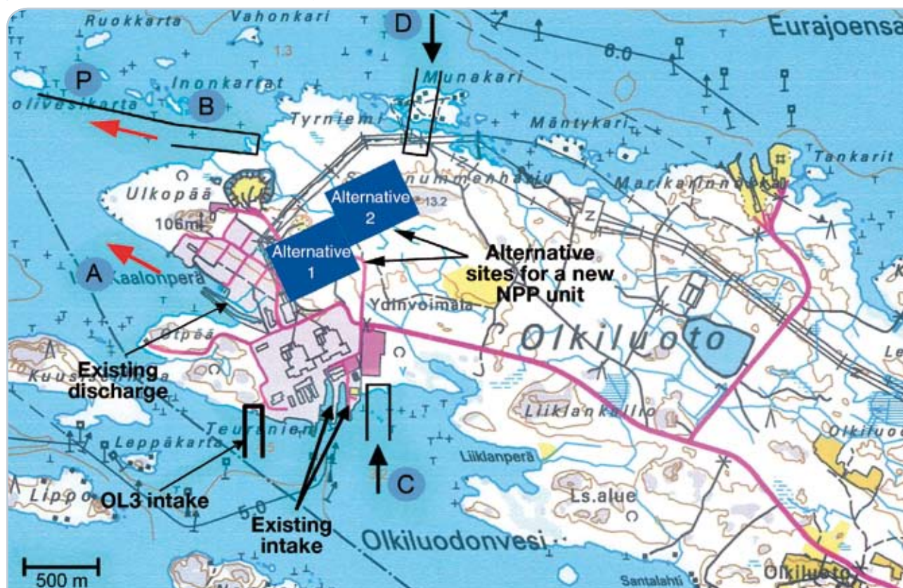
Figure 2-5 Alternative locations for the power plant unit and alternative locations for cooling water intake and discharge. A and B are locations for the cooling water discharge channel for plant unit OL4, while C and D are locations for the cooling water intake channel for plant unit OL4. P refers to a potential extension to the northern bank of discharge channel B.
