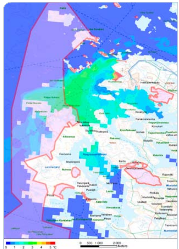
Figure 9-49 Limits of the Rauma archipelago Natura 2000 area and the spreading of cooling water at a depth of 2.5 metres during a north wind, cooling water intake at point C and discharge at point B.
