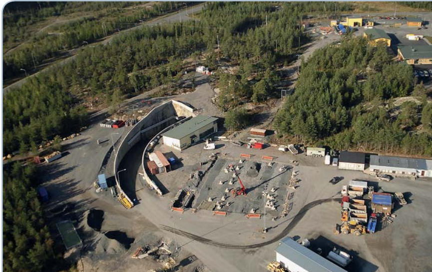
Figure 14–2 Entrance of the tunnel leading to the spent fuel final disposal research facility (ONKALO) at Olkiluoto. The research facility will eventually constitute a part of the spent fuel final repository.
