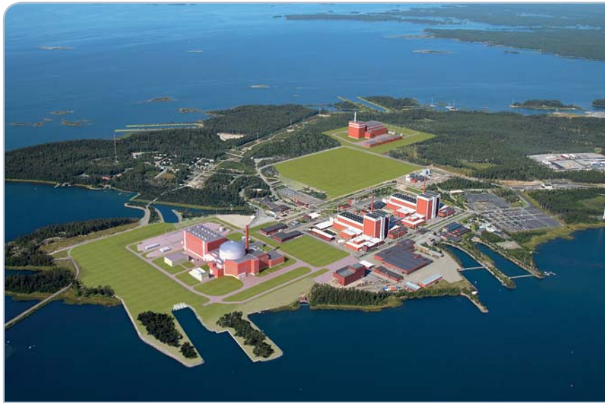
Figure 12–2 Photomontage of the Olkiluoto area in which OL4 is located at plant site alternative 2 and cooling water is taken from Eurajoki strait to the north of Olkiluoto Island and discharged to the northwest of the island.
