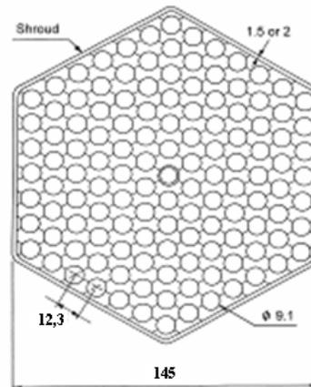
**Figure 12- Fuel assembly cross section**
