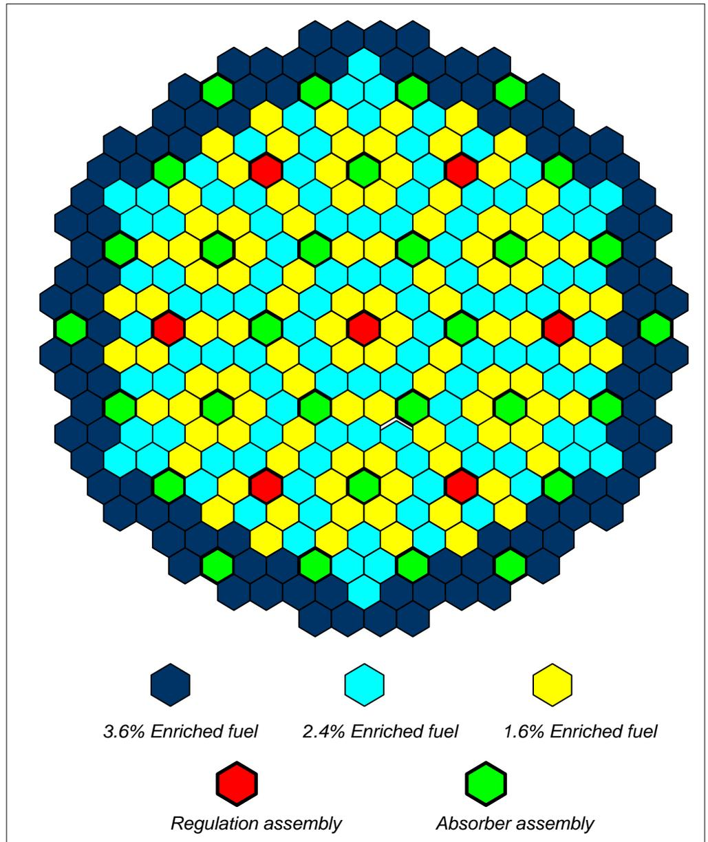
**Figure 11 - Layout of the first core for MO34**
