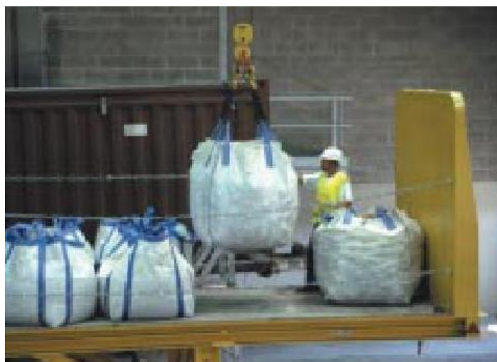
Fig. A-II. 15 Packages of VLLW of granulated structure suitable for disposal [L-110]
