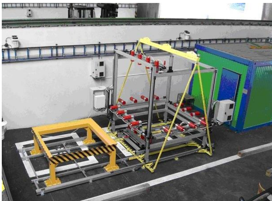
Fig. A-II. 7 Gamma scanner for the control of the radiation characteristics of FCC
