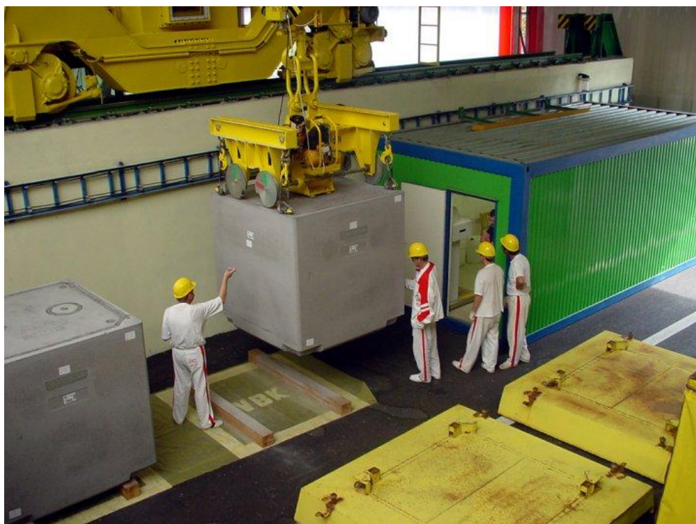
Fig. A-II. 8 Take over and preparation of FCC with VLLW for the disposal in NRR Mochovce
