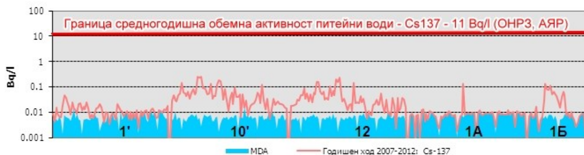
FIGURE 3.2-9: ACTIVITY OF 137 Cs (Bq/L) IN THE WATERS FROM HFS OF KOZLODUY NPP, 2007 ÷ 2012
