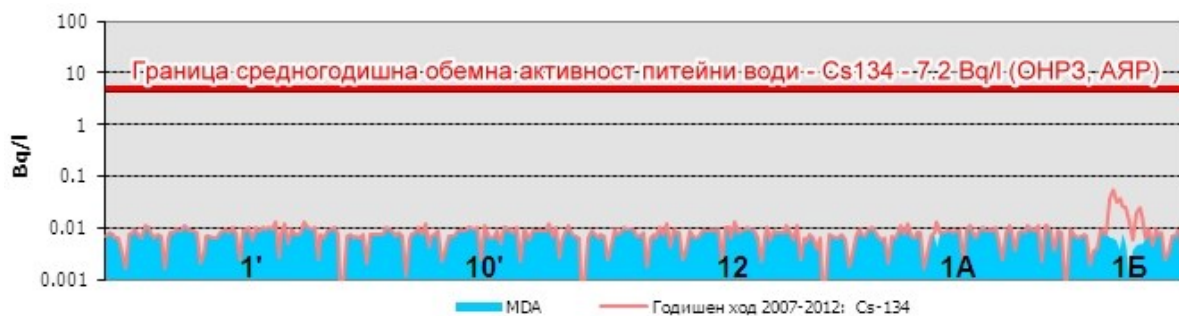
FIGURE 3.2-8: ACTIVITY OF 134 Cs (Bq/L) IN THE WATERS FROM HFS OF KOZLODUY NPP, 2007 ÷ 2012
