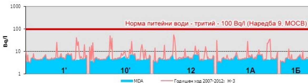
FIGURE 3.2-6: ACTIVITY OF 3 H (BQ/L) IN THE WATERS FROM HFS OF KOZLODUY NPP, 2007 ÷ 2012
