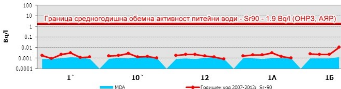
FIGURE 3.2-7: ACTIVITY OF 90 Sr (Bq/L) IN THE WATERS FROM HFS OF KOZLODUY NPP, 2007 ÷ 2012
