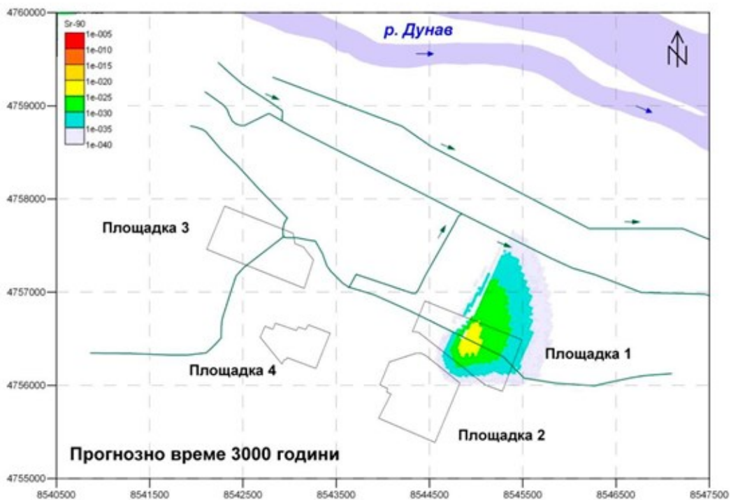
FIGURE 4.2-34: FORECAST MIGRATION OF 90 Sr ISOTOPE AT PROJECTED TIME OF 1000 AND 3000 YEARS AFTER ITS ENTRY INTO THE GROUNDWATER IN THE REGION OF SITE 2. MIGRATION MODEL MM-4
