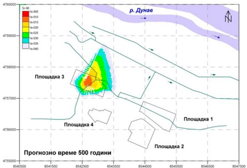
FIGURE 4.2-38: FORECAST MIGRATION OF ^{90}\text{Sr} ISOTOPE AT PROJECTED TIME OF 100 AND 500 YEARS AFTER ITS ENTRY INTO THE GROUNDWATER IN THE REGION OF SITE 3. MIGRATION MODEL MM-6
