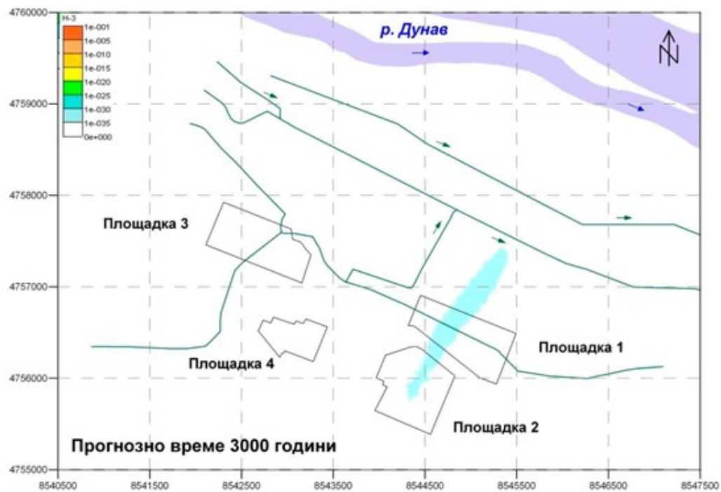
FIGURE 4.2-32: FORECAST MIGRATION OF ^3\text{H} ISOTOPE AT PROJECTED TIME OF 1000 AND 3000 YEARS AFTER ITS ENTRY INTO THE GROUNDWATER IN THE REGION OF SITE 2. MIGRATION MODEL MM-3
