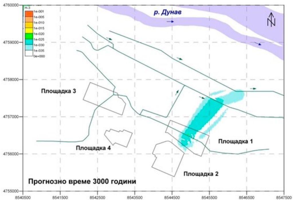
FIGURE 4.2-27: FORECAST MIGRATION OF ^3\text{H} ISOTOPE AT PROJECTED TIME OF 1000 AND 3000 YEARS AFTER ITS ENTRY INTO THE GROUNDWATER IN THE REGION OF SITE 1. MIGRATION MODEL MM-1
