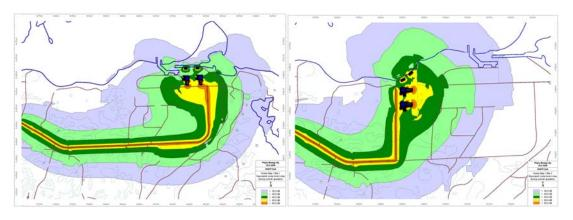
Figure 5.7-2. Noise map for Site No. 1 and Site No. 2 during operation phase.
