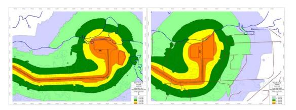
Figure 5.7-1. Noise map for Site No. 1 and Site No. 2 during construction phase.
